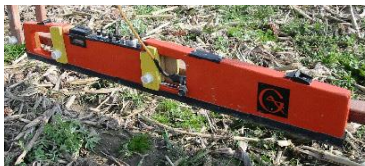
Figure 8 Non-contact electromagnetic sensor for soil mapping 33
