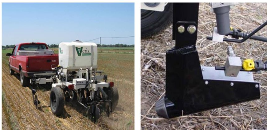
Figure 5 Electrochemical sensor for soil pH mapping 28,29
